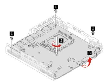
The failing system board must be returned with a microprocessor socket cover to protect the pins during shipping and handling.
