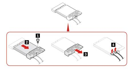
Note: While installing, ensure that you connect the gray cable to the connector labeled 1 (auxiliary) and the black cable to connector labeled 2 (main) on the card.
