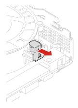
4. Disconnect the system fan cable from the system fan connector on the system board.
