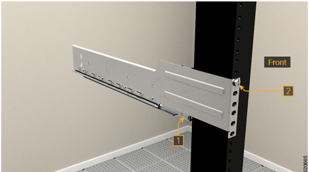
Figure 31: Two Post Slider Integration in the 19" Rack
