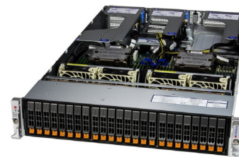
Supermicro® Hyper A+ Server AS -2125HS-TNR 10 (used with permission from Super Micro Computer, Inc.)
