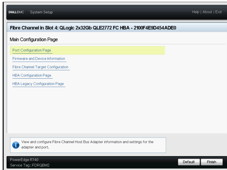
Figure 3-12. Dell System Setup: Main Configuration
