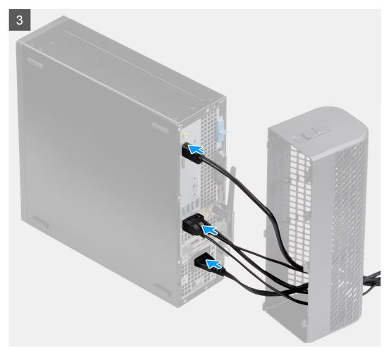
$\textbf{3.} \ \ \text{Align the cable cover retaining hooks into the slots on the OptiPlex 5090 Small Form Factor chassis.}$
