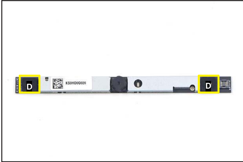
Figure 3-58. Camera Module Removal
