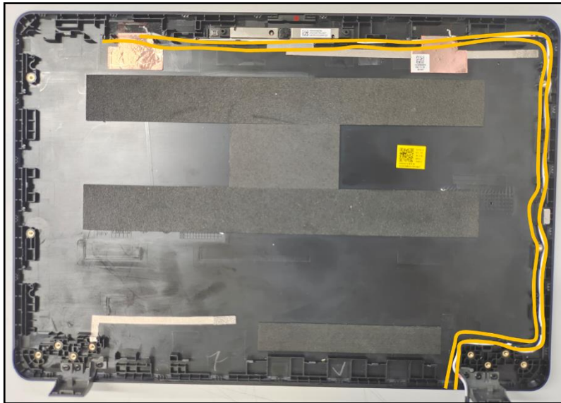
Figure 3-62. WLAN Antenna Removal
