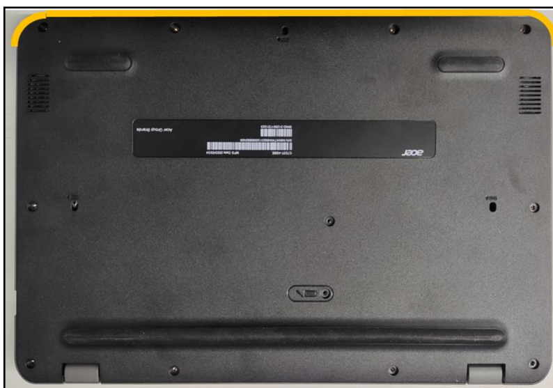
Figure 3-4. Base Cover Removal
