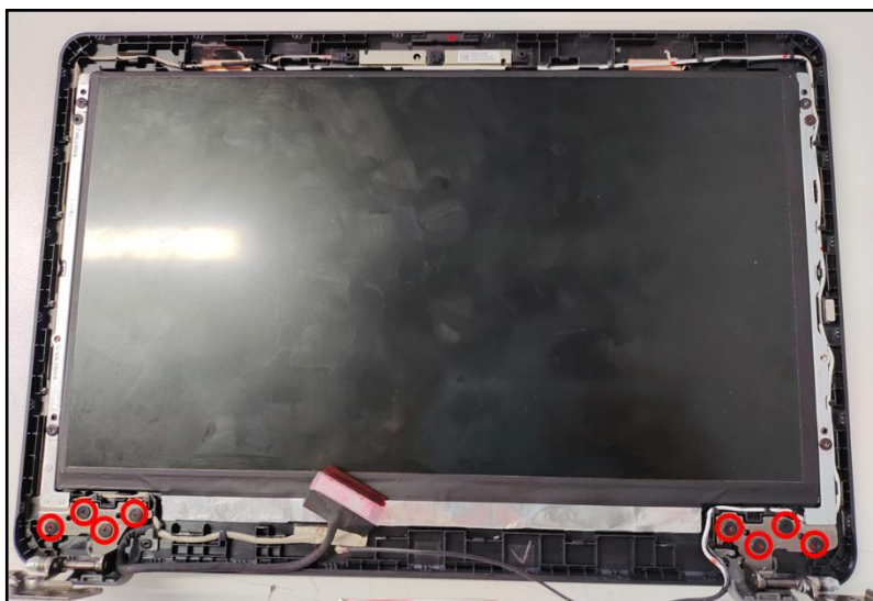
Figure 3-49. LCD Hinges Removal
