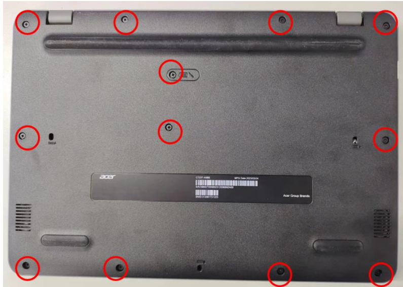
Figure 3-120. Replacing the Base Cover
