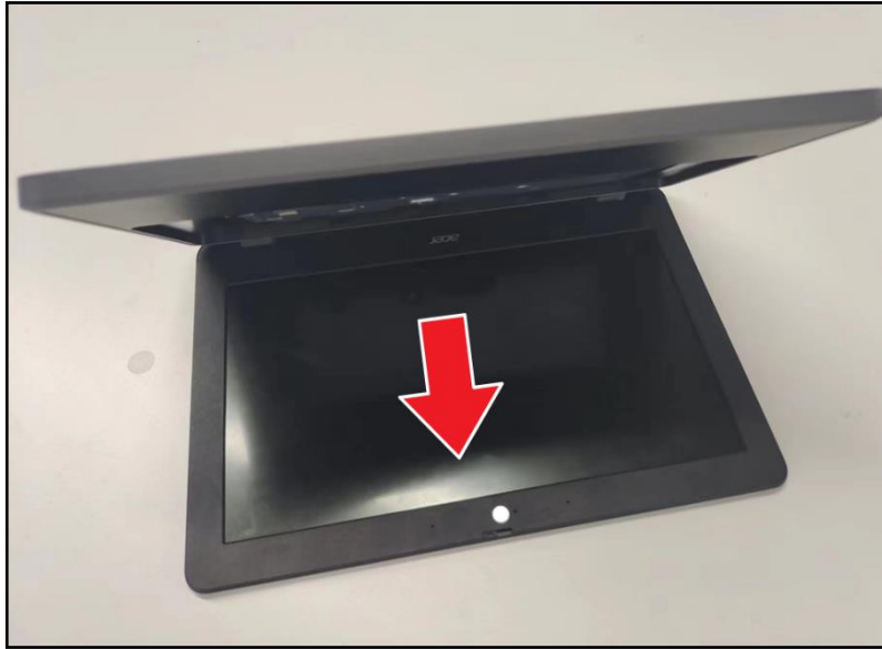
Figure 3-33. LCD Module Removal
