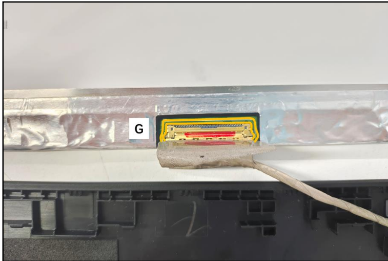
Figure 3-52. eDP Cable Removal
