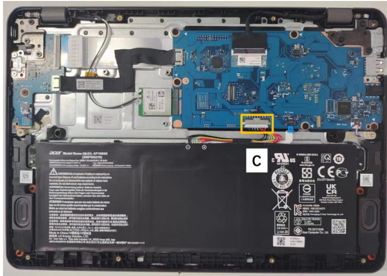
Figure 3-115. Replacing the Battery Pack
