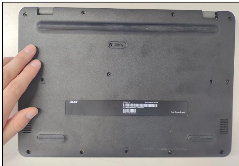
Figure 3-119. Replacing the Base Cover
