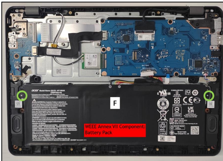
Figure 3-9. Battery Pack Removal
