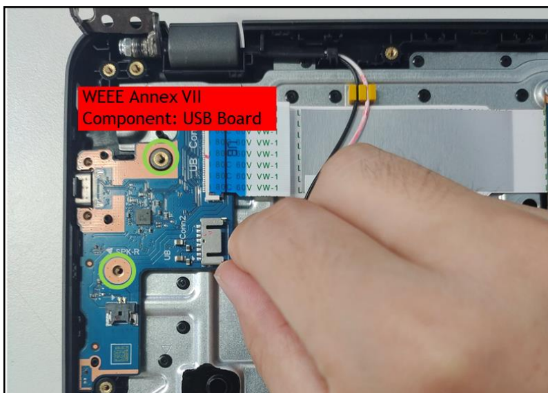
Figure 3-27. USB Board Removal
