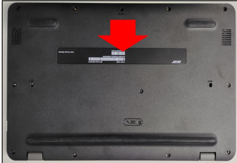
Figure 3-5. Base Cover Removal
