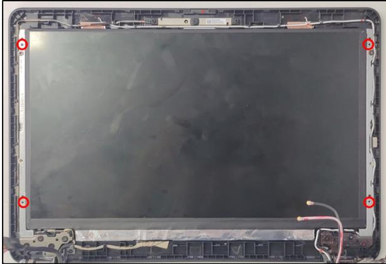
Figure 3-80. Replacing the LCD Panel
