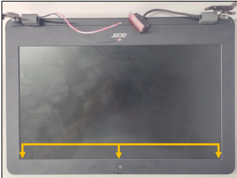
Figure 3-43. LCD Panel Removal
