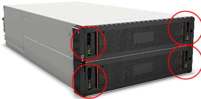
Figure 2-10 Drawer Sideplane Status panel locations
