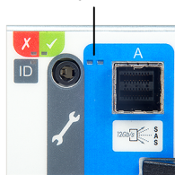
Figure 2-9 I/O module SAS Activity LED location
