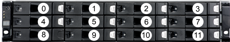
Figure 2-2 Veritas 2U12 65.5TiB/72TB Storage Shelf disk drive slot layout
