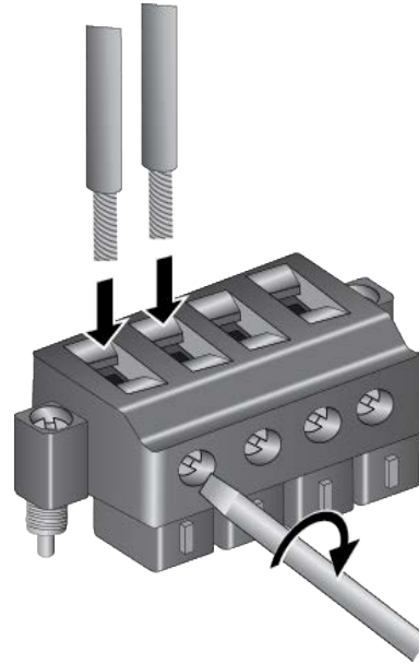
Figure 52. Inserting Wires into the DC Input Plug
