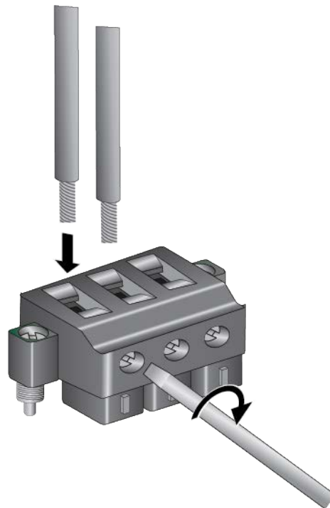
Figure 44. Inserting the Wires into the Alarm Out Plug
