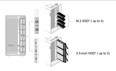
Note: M.2 SSD installation priority is higher than 3.5-inch HDD.
