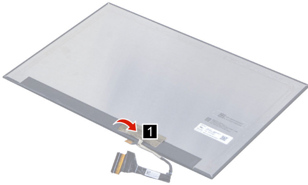
Figure 60. Peel off the tape
