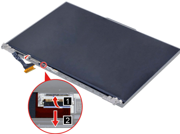
Figure 58. Disconnect the EDP cable from the sensor board and release the EDP cable
