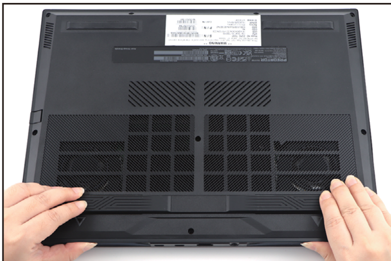
Figure 1-4. Base Cover Removal
