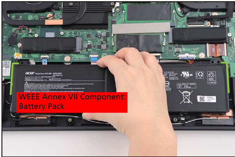
Figure 1-8. Battery Pack Removal
