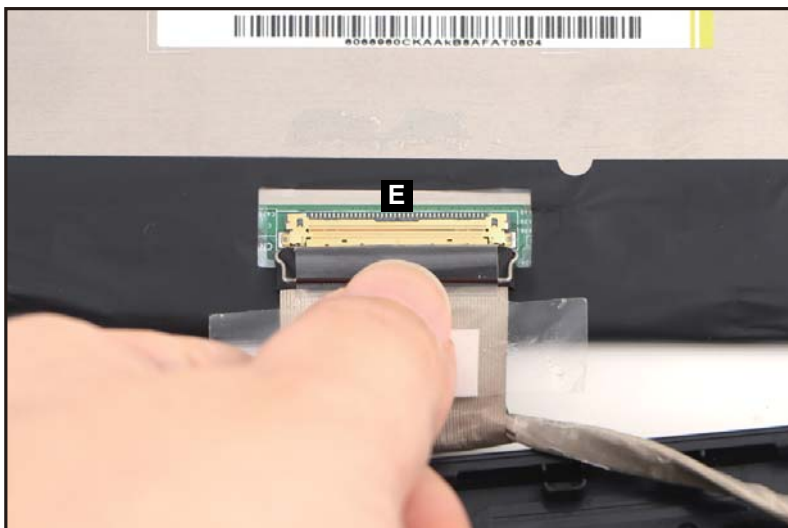
Figure 1-48. LCD Panel Removal
