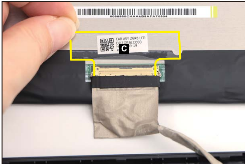
Figure 1-46. LCD Panel Removal
