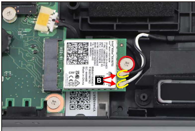
Figure 1-20. WLAN Module Removal
