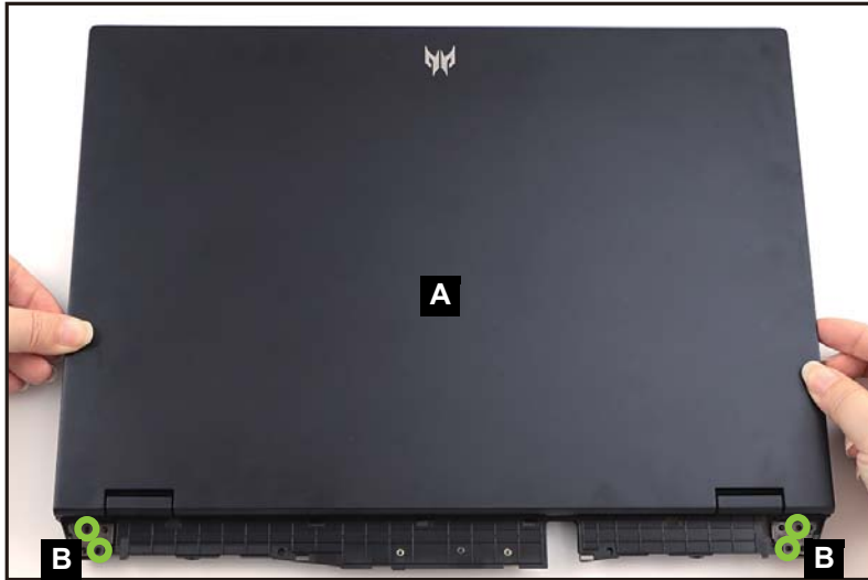
Figure 1-38. LCD Module Removal
