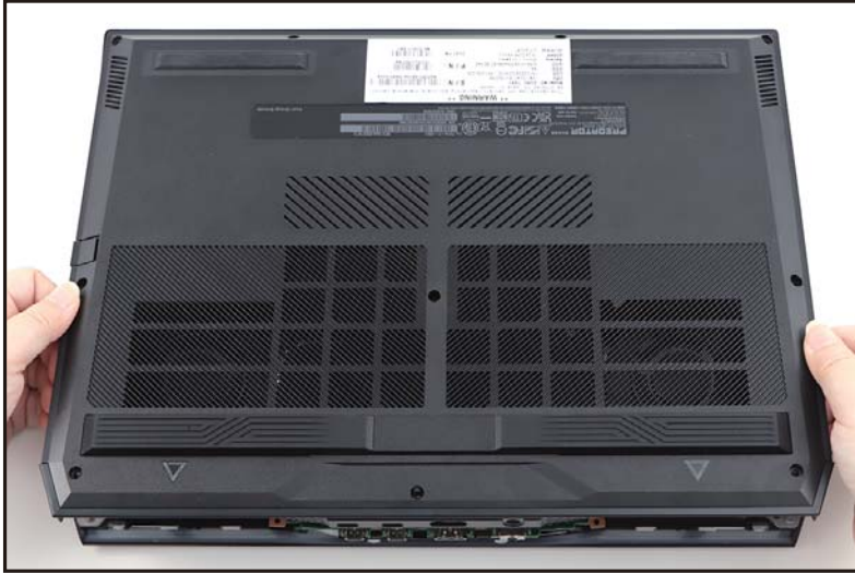
Figure 1-5. Base Cover Removal
