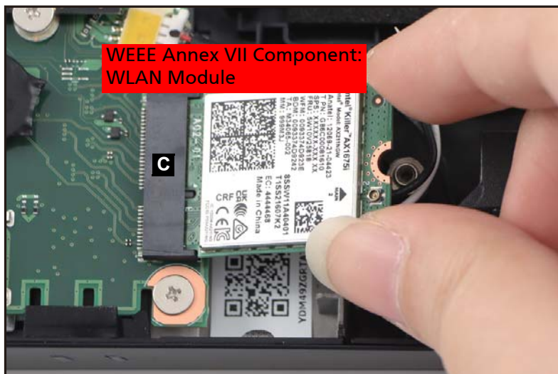
Figure 1-21. WLAN Module Removal
