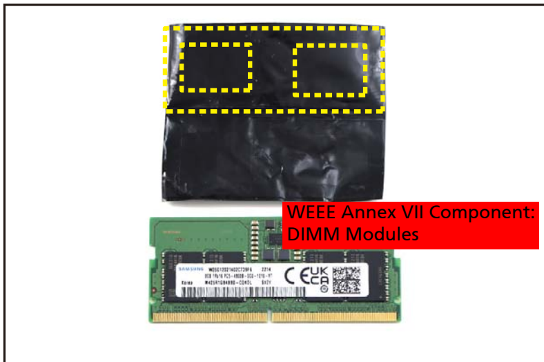
Figure 1-18. DIMM Module Removal
