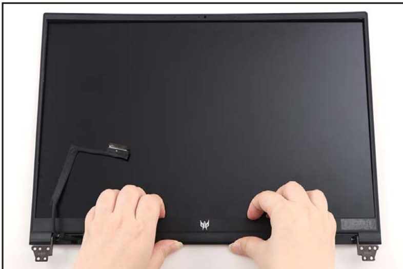
Figure 1-43. LCD Bezel Removal
