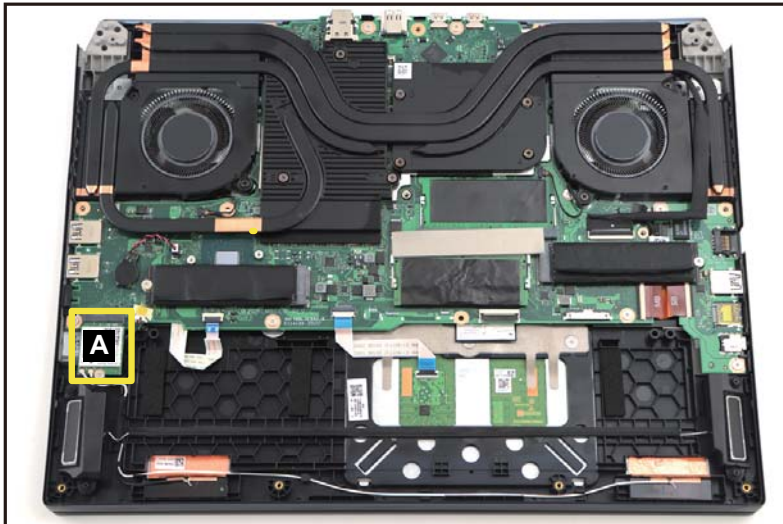
Figure 1-19. WLAN Module Location
