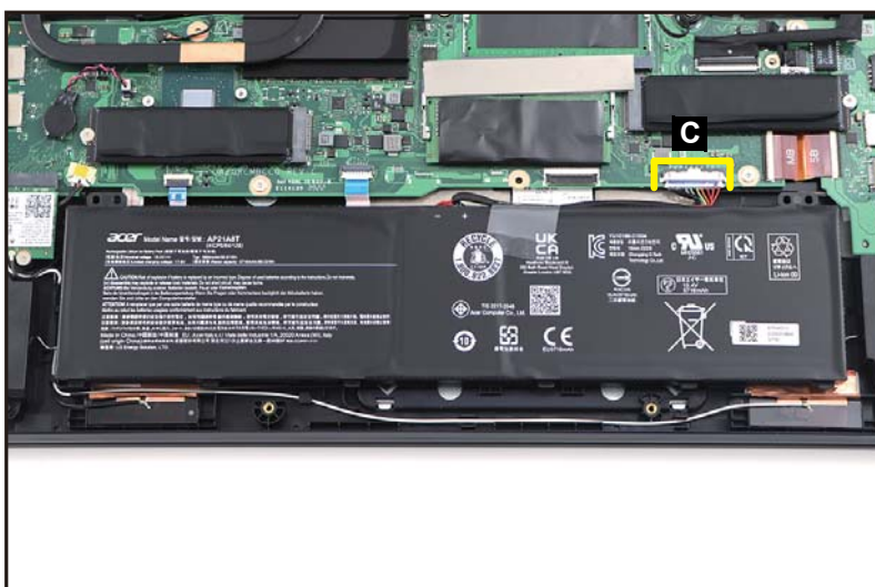
Figure 1-7. Battery Pack Removal
