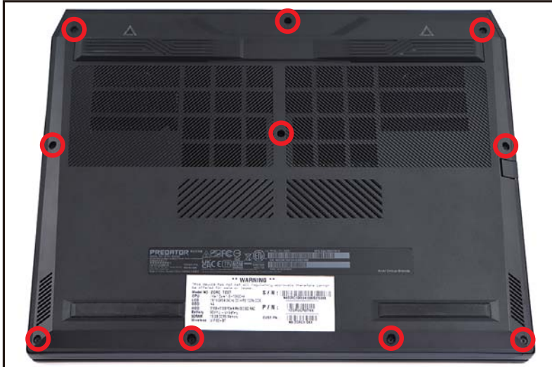
Figure 1-3. Base Cover Removal
