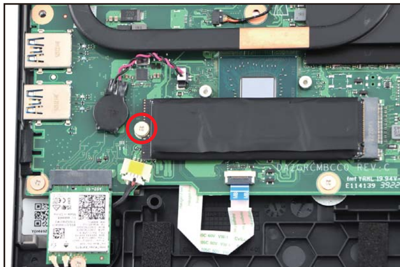
Figure 1-10. SSD Module Removal
