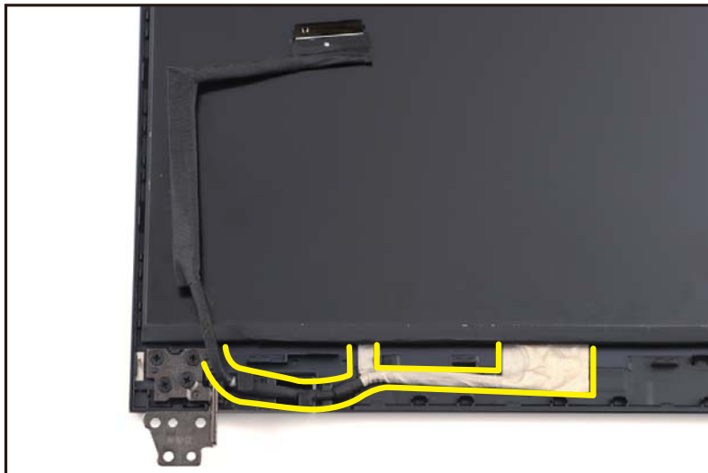
Figure 1-44. LCD Panel Removal
