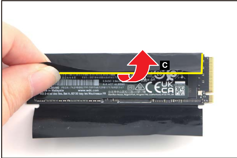
Figure 1-13. SSD Module Removal
