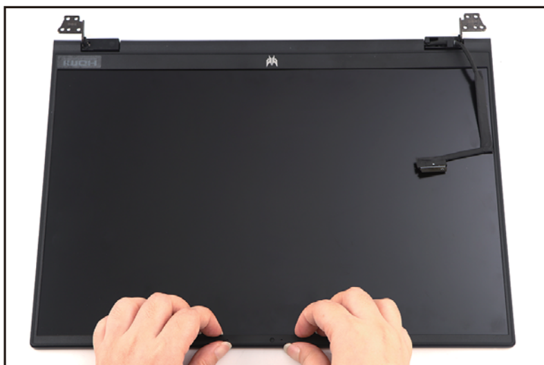
Figure 1-40. LCD Bezel Removal
