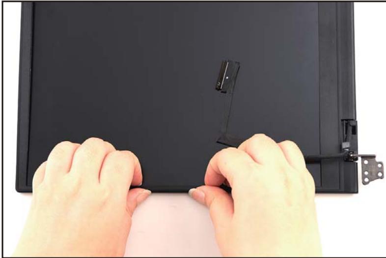
Figure 1-42. LCD Bezel Removal
