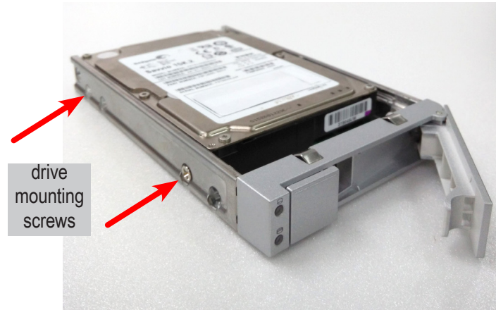
2.5" drive carrier with HDD installed, front view
