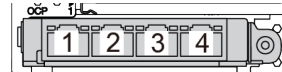
Figure 9. Ports on the OCP 3.0 Ethernet adapter (four connectors, seen from the rear)
