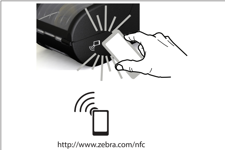
Figure 31 • Near Field Communication (NFC) Pairing
