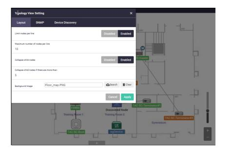
From the **Layout** tab you can optionally set up an existing network topology to do things like: limit the nodes that appear per line, set a maximum number of nodes per line, collapse the child nodes or add a background image. A child node is a node that is connected to a node above it (a parent node). The example above shows a layout floor map that has been added.
