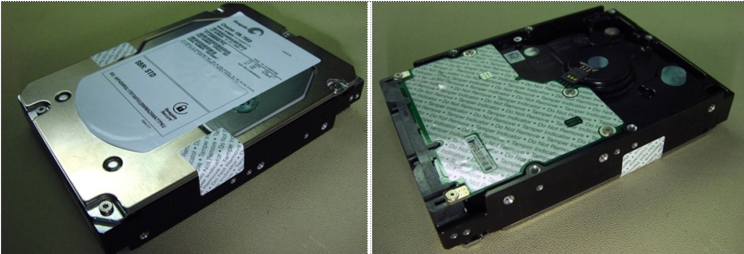
Figure 10. Example of FIPS tamper evidence labels.
