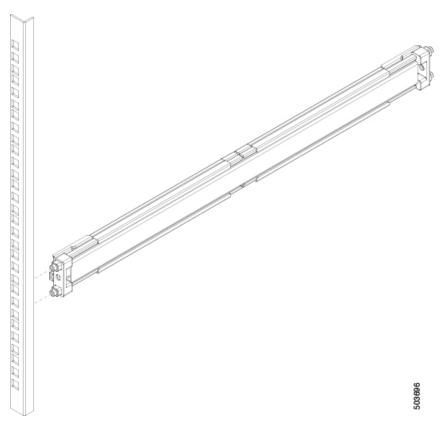
**Step 3** Fasten the two outer rails to the front posts of the rack by pushing the latch into place, as shown in the following illustration:
