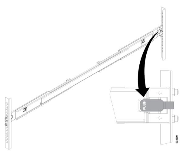
**Step 6** If installing from the front of the rack, slide the chassis into the rack by aligning the inner rails into the outer rails, and sliding the chassis back until the front panel is flush with the front of the rack. Then secure the retainer screws on the inner rails into the rack, as shown in the following illustration:
