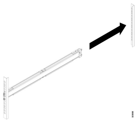
**Step 5** Fasten the two outer rails to the back posts of the rack by pushing the latch into place, as shown in the following illustration:
