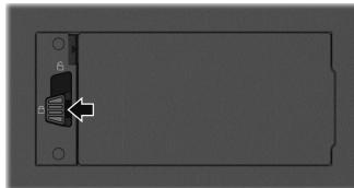
**CAUTION:** Make sure the battery latch is correctly locked, not revealing the underneath red part.
