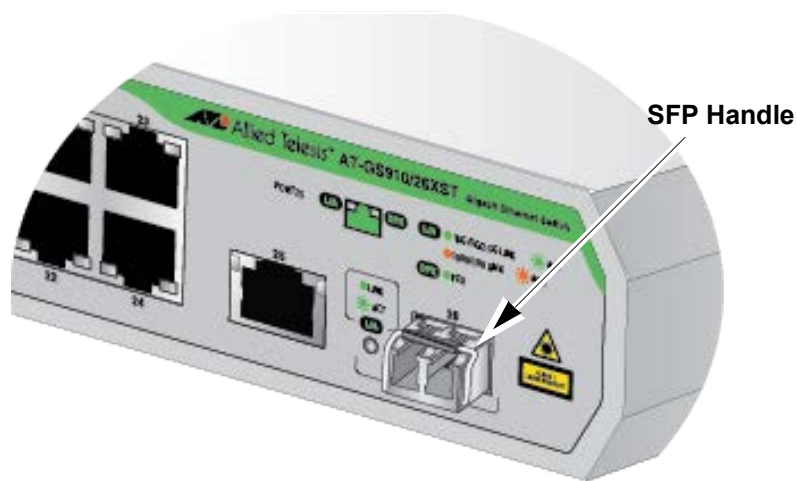
Figure 22. Positioning the SFP Handle Upright
