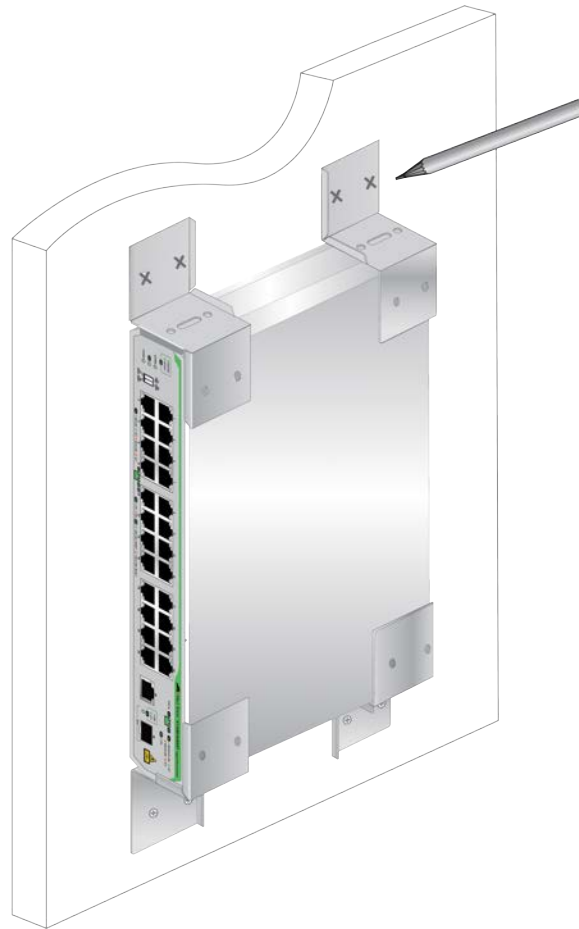
Figure 28. Marking the Screw Hole Locations for the Top Brackets
