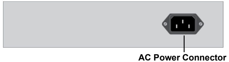
Figure 5. Rear Panel for the GS910/10XST Switch
