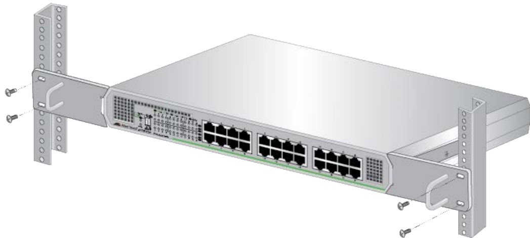
Figure 35. Attaching the Switch to Equipment Rack
