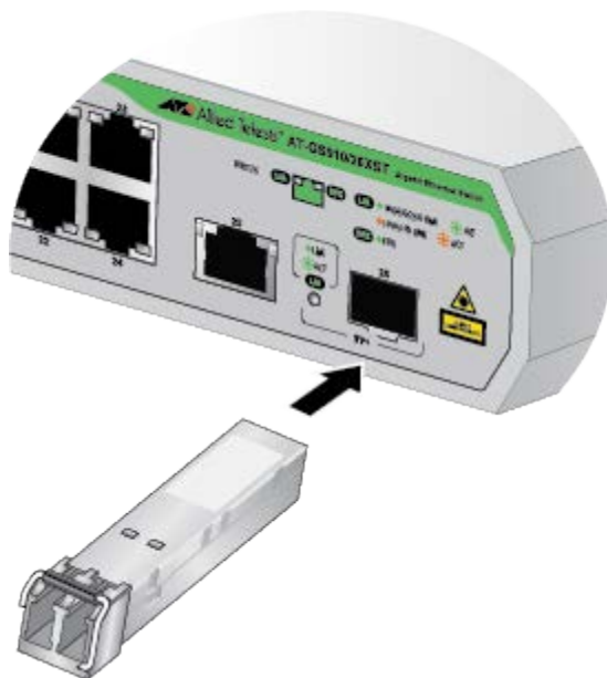
Figure 21. Installing an SFP Transceiver
