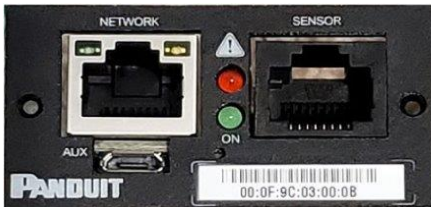
Figure 1: Ethernet Port for Network Connection
