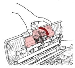
b. Slightly pull out the brake roller to release the left side of the shaft, and then pull out the right side of the shaft from the hole.
