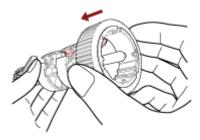
b. Insert the retaining clip of the other pick roller into the slot.
