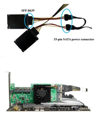
Connect the remaining NVMe SSDs to the SSD7580B controller as described above. Once complete, Power on the system.
