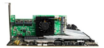
Connect two pieces of NVMe with SFF-8639 port, and connect SFF-8654 port to SSD7580A. Connect the 15-pin SATA power connector to the system's power supply.
