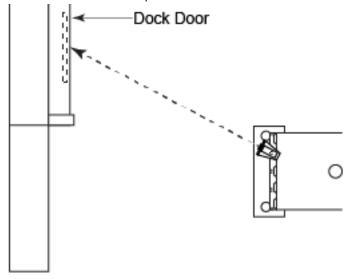
**3.** Connect the photo eye cable to the quick connect on the rear of the A-panel closest to the dock door.
