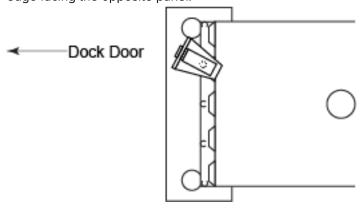
2. Adhere the reflective tape to the inside of the dock door at the same level as the photo eye lens.
