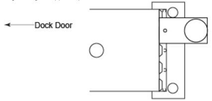
2. Connect the stack light cable to the quick connect on the rear of A-panel farthest from the dock door.
