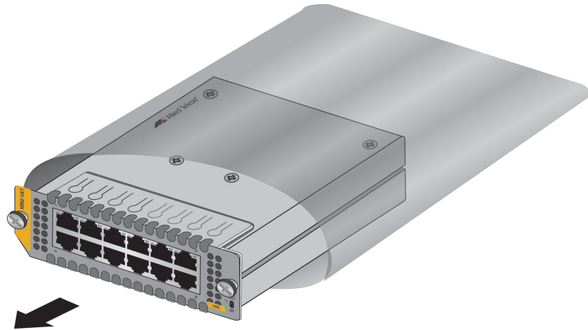
Figure 55. Removing the Ethernet Line Card from the Anti-static Bag
