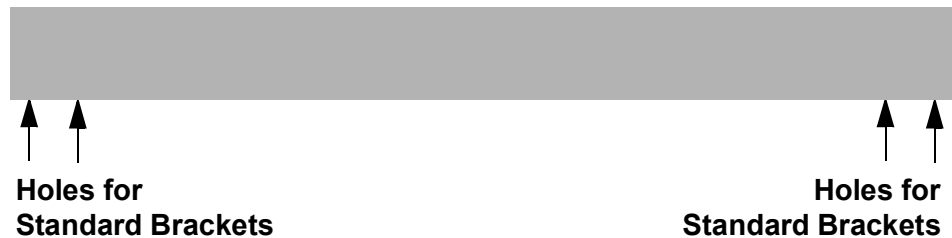
Figure 64. Holes for the Equipment Rack Brackets on the x950-28XSQ and x950-28XTQm Switches
