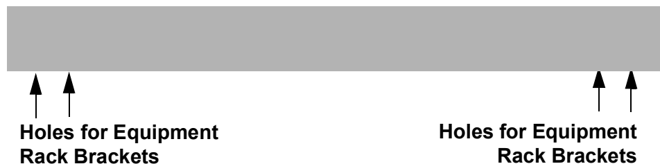
Figure 65. Holes for the Equipment Rack Brackets on the x950-52XSQ and x950-52XTQm Switches
