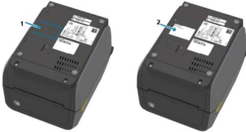
Figure 5 Label Locations for Thermal Transfer Printers
