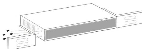
Use the screws provided with the equipment rack to mount the Intellinet Network Solutions data switch on the rack.
