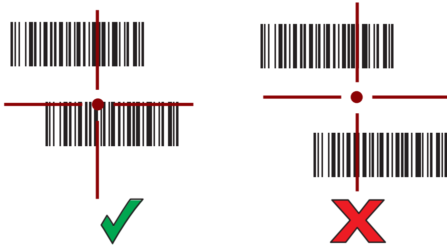
Figure 18 Pick List Mode with Multiple Barcodes - Standard Range
