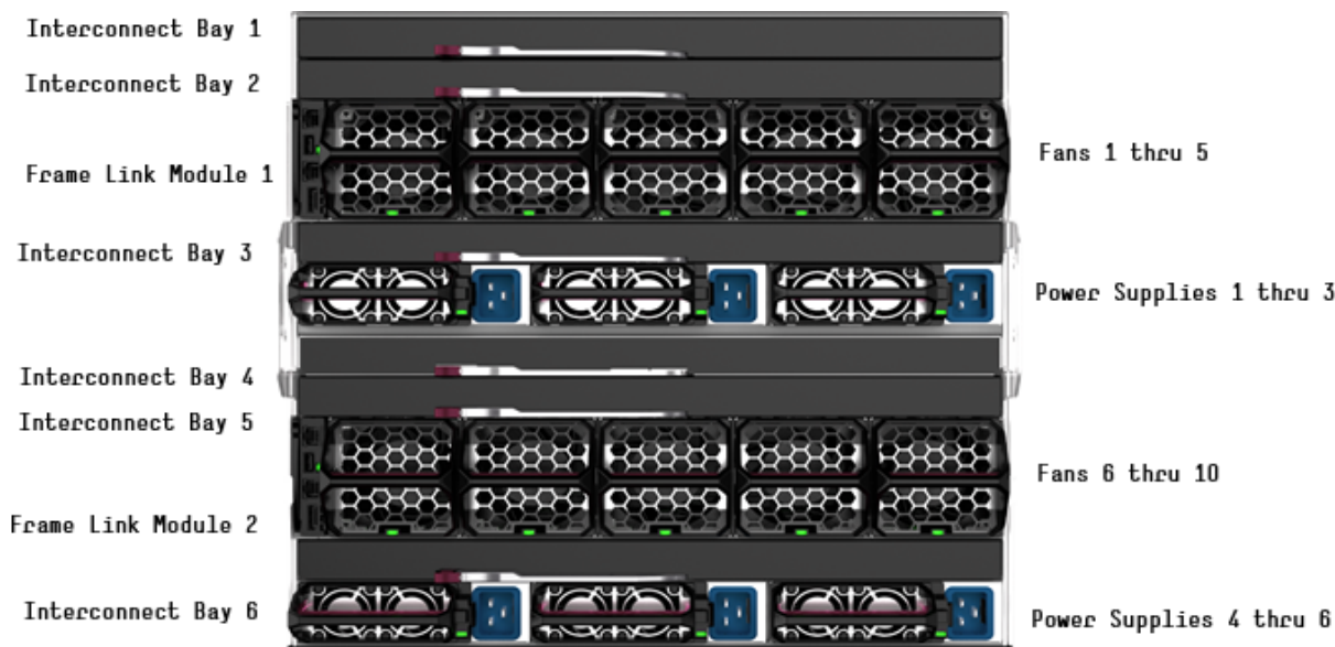
HPE Synergy 12000 Frame - Rear View
