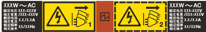
Figure 72. Hot-swap power supply label on the cover
