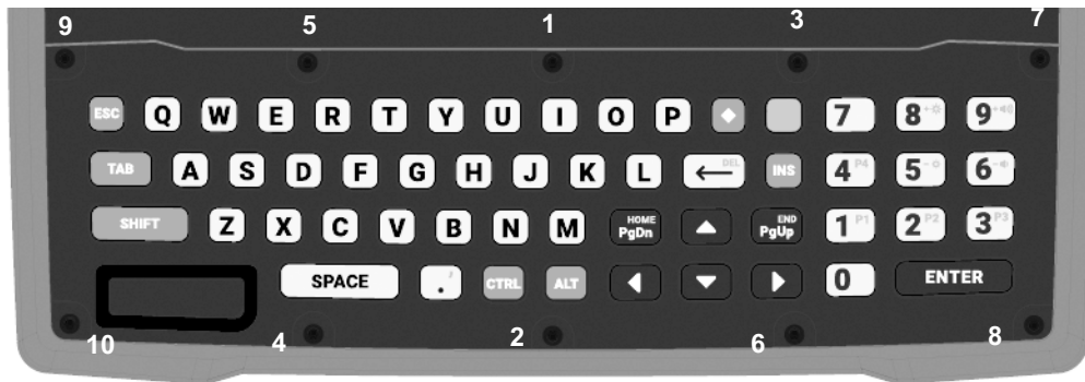
Figure 3 Bezel Screw Torque Sequence
