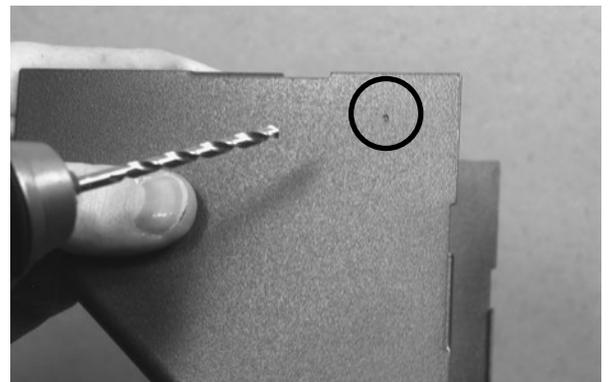
**2** Install Tamper Resistant Screw through drilled hole in the Cover into the tab with hole on the Fitting Base.
