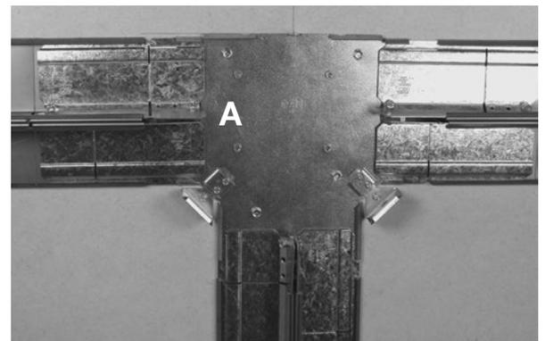
**NOTE: The DS4015 Tee Fitting can be configured two different ways depending on where the communication cables are installed. Electrical wiring is meant to be housed inside the Internal Tunnel. Communication cables are controlled by the Radius Control Inserts.**
