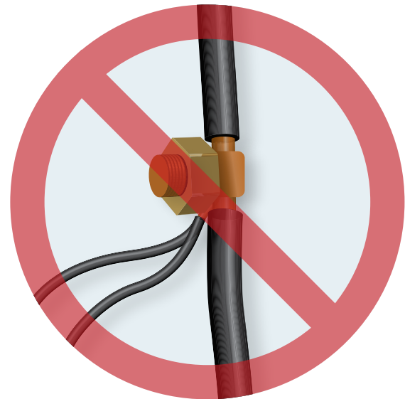
Figure 2 Terminating both sensor leads at the same point may result in inaccurate AVT results.
