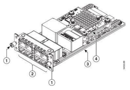
1 Screws 2 Ports 3 Network interface module 4 PVDM4
