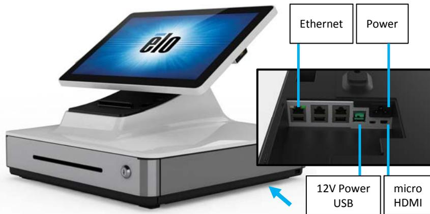
Connect power and ethernet cable. Connections are underneath the register near the back. Before plugging or unplugging the micro-HDMI cable, first unplug the power cable.
