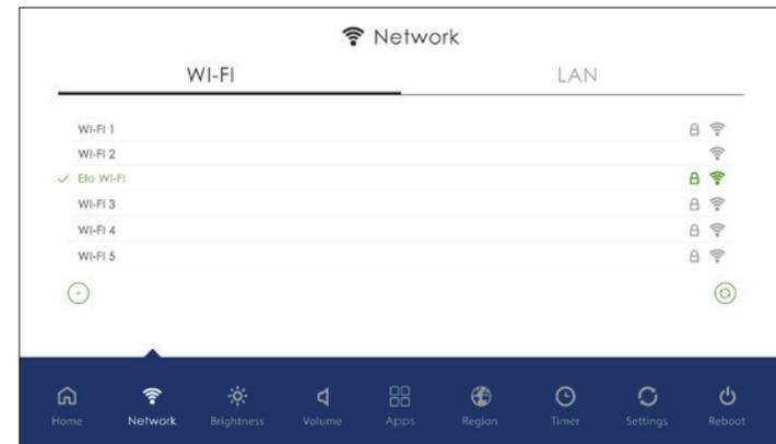
If an Internet connection is not found in Step 3, hold the power button for 3 seconds and release. This lets you enter the set-up page to find your Wi-Fi connection. Under the Network Tab, select the Wi-Fi network. Once connected, your device should start auto provisioning itself to your software provider. Once set up is complete, password **1elo** can be used to re-enter control panel if needed.
