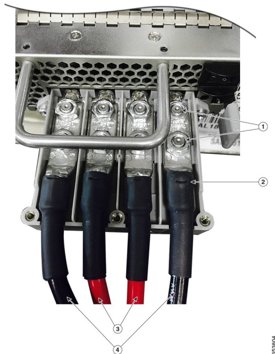
Figure 41: Connecting Cables to the Terminal Slots
