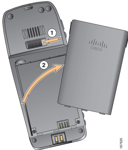
Figure 3-1 Removal of Cover to Install the Battery
