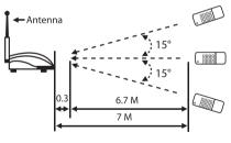
Distance not less than 0.3 M and not more than 7M Working angle not more than +/- 15°
