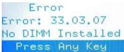
Figure 6: Error message: 33.03.07 No DIMM Installed
