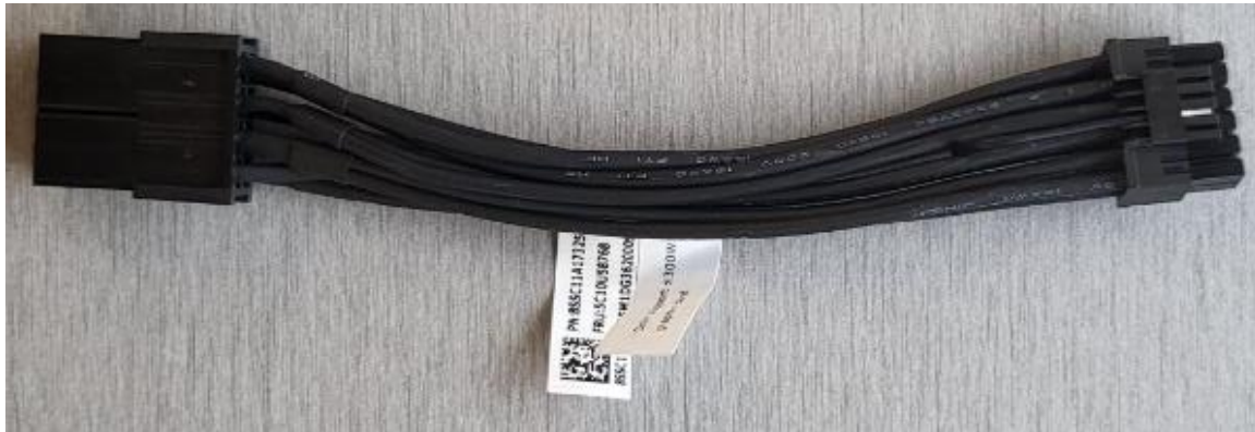
8-pin (female) to 12VHPWR (male) Power Cable (FRU# 5C10U58768)
