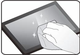
Clean the screen thoroughly with the screen cleaning cloth (included). Make sure there is not any dust, lint, fingerprints, or other particles on the screen surface.
