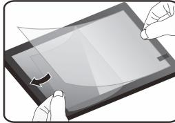
Align the film (adhesive side facing down) with the screen edge and attach the exposed part of the film to the screen. Continue across the screen while peeling off the backing layer a little at a time.
