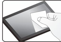
Use the applicator (included) to smooth the film as you work your way across the screen. Remove any remaining air bubbles by pushing them toward the outer edge of the film with the applicator.
