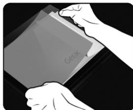
Align the film (adhesive side facing down) with the screen edge and attach the exposed part of the film to the screen. Continue to apply across the screen while peeling off the backing layer a little at a time.
