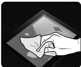
Clean the screen thoroughly with the special cleaning cloth (supplied with your computer). Make sure there is not any dust, lint, fingerprints, or other particles on the screen surface.
