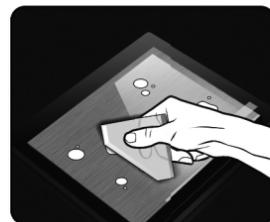
Use the applicator (included) to smooth the film as you work your way across the screen. Remove any remaining air bubbles by pushing them toward the outer edge of the film with the applicator.
