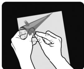
Pull the transparent tab to peel the backing layer off the film about 1½ inch along one edge. Do not peel off the entire piece at one time.
