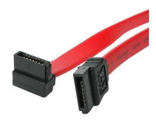
The SATA18RA1 Right Angle (90-degree) SATA Cable features a standard (straight) SATA receptacle as well as a right-angled SATA receptacle, providing a simple 18-inch connection to a Serial ATA drive, with full SATA 3.0 bandwidth support of up to 6Gbps when used with SATA 3.0 compliant drives.
