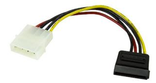
This 6in 4 Pin LP4to SATA power adapter cable features one 4 Pin LP4 male connector and one female SATA power connector, allowing you to power a Serial ATA hard drive from a conventional LP4 connection, eliminating the need to upgrade the computer power supply for compatibility with the SATA hard drive.
