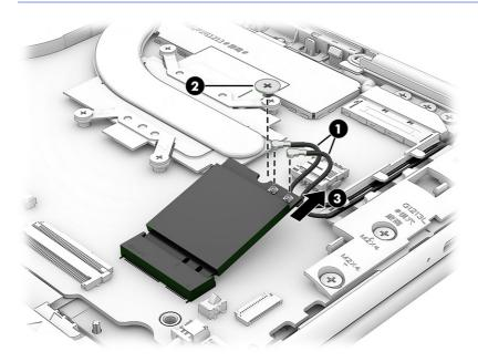
3. If the WLAN antenna is not connected to the terminal on the WLAN module, install a protective sleeve on the antenna connector, as shown in the following illustration.
