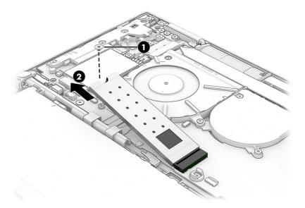
3. Remove the protective sleeve from the solid-state drive.
