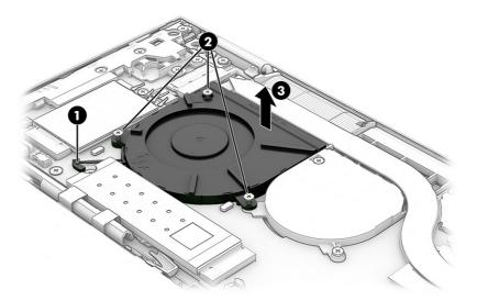
3. Loosen the two captive Phillips screws (1) that secure the dummy fan to the computer, and then remove the dummy fan from the computer (2).
