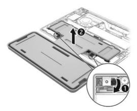
i. Rotate the battery up and over into the cavity of the containment tray.
