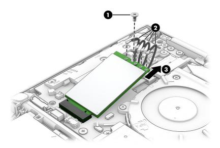
4. If the WWAN antenna is not connected to the terminal on the WWAN module, a protective sleeve must be installed on the antenna connector, as shown in the following illustration.
