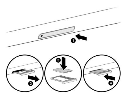
To remove the nano SIM card, insert a small straightened paper clip or a SIM card ejector pin into the card tray access hole to remove the tray. Remove the nano SIM card. Replace the tray in the computer and press in gently on the tray until it is firmly seated.
