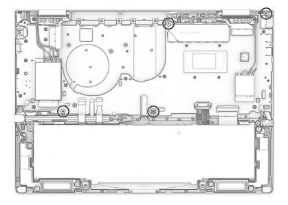
3. Carefully lift the left side of the system board (1), and then slide it out (2).
