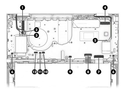
2. Remove the four Phillips M2.0  $\times$  5.0 screws that secure the system board to the computer.
