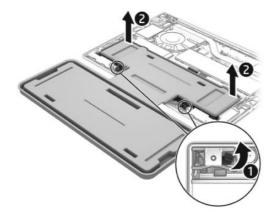
e. Connect the battery cable to the system board. The connector location might vary.
