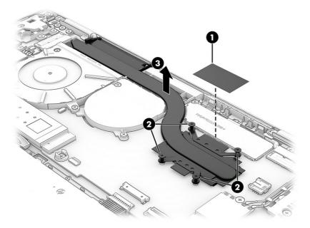
4. Thoroughly clean the thermal material from the surfaces of the heat sink and the system board components each time the heat sink is removed. Replacement thermal material is included with the heat sink and system board spare part kits. The following illustration shows the replacement thermal material locations.
