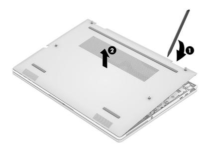
To replace the bottom cover, reverse the removal procedures.
