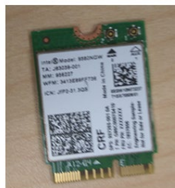
Wireless Module PCB
