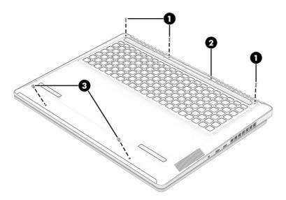
5. Insert a tool (1) into the seam near the captive screw (2), and then release the bottom cover (3).
