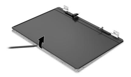
b. Use a heat gun to heat both sides of the display rear cover with the OMEN logo in the middle to approximately  $60^{\circ}$  C ( $140^{\circ}$  F).
