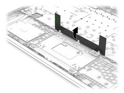
2. Remove three Phillips M2.0 × 3.0 screws (1) that secure the plastic bracket to the touchpad, and then remove the bracket (2).
