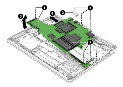
5. If you are replacing the system board, install the USB bracket you removed onto the new board.
