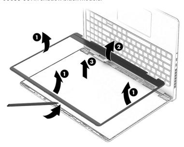
NOTE: When removing the bezel, do not pull up the black protective strip under the bottom of the bezel. Be sure the strip remains flat against the panel.
