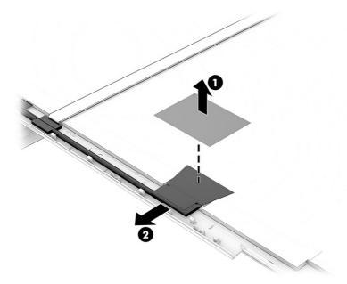
j. When installing a display panel, be sure to install the stretchable tape on the left and right sides of the display back cover as shown in the following illustration.
