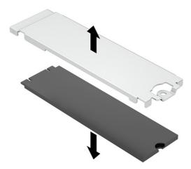
When installing a drive, be sure a thermal pad is installed on the bottom side of the bracket.
