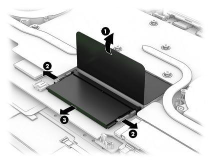
To protect a memory module after removal, place it in an electrostatic-safe container.
