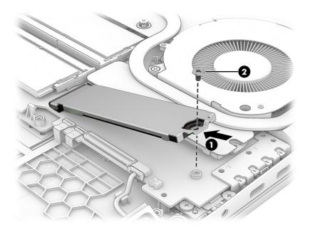
NOTE: SSDs are designed with a notch to prevent incorrect insertion.
