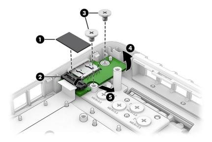
To install the USB board, reverse this procedure.
