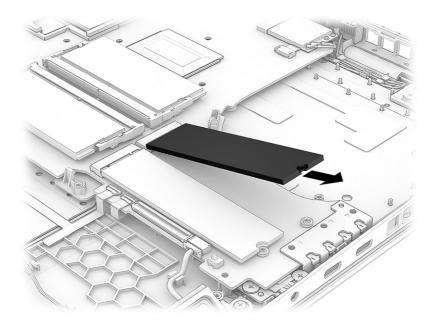
To install the SSD, reverse the removal procedures.
