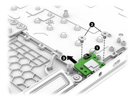
To install the audio board, reverse this procedure.
