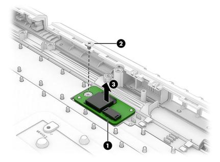
To install the ULL board, reverse this procedure.
