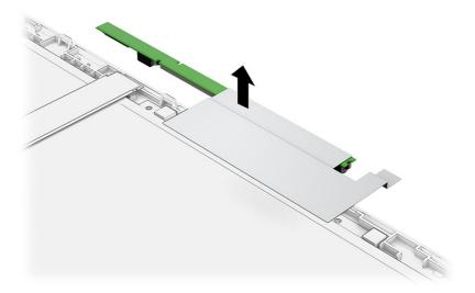
g. Remove the tape (1) from the OLED board, and then disconnect the white flat cable (2) from the
