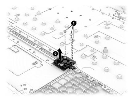
3. Remove the four Phillips M2.0 × 2.5 screws (1) that secure the metal bracket to the computer, and then remove the bracket (2).
