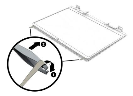
e. Lift the top of the panel (1) up, and then pull the bottom of the panel (2) away from the display rear cover.
