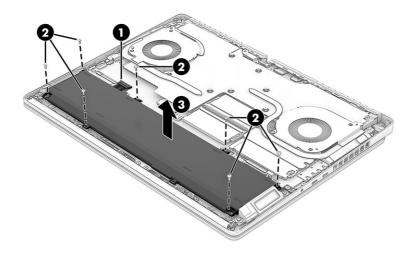
To install the battery, reverse the removal procedures.
