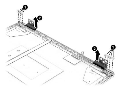
c. Remove the hinge covers by removing the Phillips M2.0 × 3.0 screw (1) from each cover, and then sliding the covers (2) off the hinges. Note the rubber pieces (3) that are installed inside the hinge covers. Be sure to install the rubber pieces when reassembling the hinge covers.
