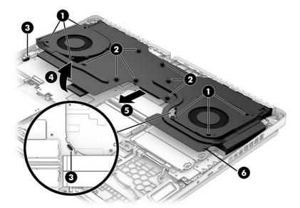
6. Each time the heat sink is removed, thoroughly clean and replace the gray thermal grease (1) and white thermal grease (2) from the surface of the heat sink and system board. You do not need to replace the thermal pads (3). Different thermal modules are available depending on processor and graphics. The primary SSD cover is soldered on the thermal module only on models with 5070Ti, 5080, and 5090 graphics.
