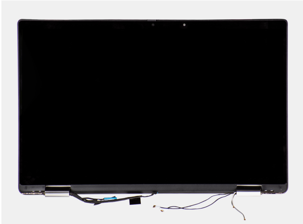
Figure 5. Display assembly with antennae cables
