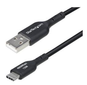
Charge a USB Type-C mobile device or transfer files to a USB-A host computer with this high-quality USB-A to Type-C cable. The USB-A to USB-C charger cord supports up to 15W and 3A output for fast charging. It supports USB 2.0 (480Mbps) transfer rates and is suitable for general use.
