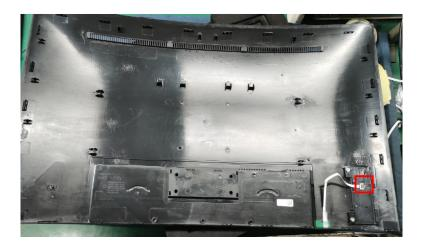
3. Use a screwdriver to tighten the key board to rear cover.
